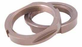
**Lockrings**: An essential part of fixy bikes, the lockring is designed to work with either the Victoire rear hub or any track hub that use the 1.29X24 TPI left thread. Both strong and light, the Victoire lockring is larger than most models available on the market. Made with 7075-T6 alloy, it is 7mm thick, anodized to improve stiffness and can be locked with a lockring wrench or a 36mm wrench.
